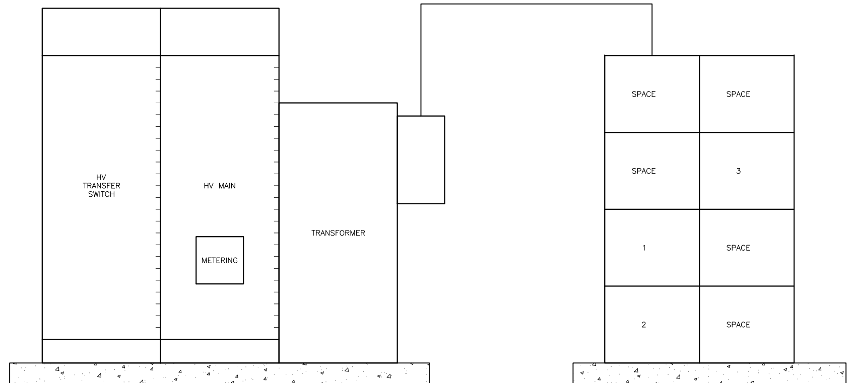
SUBSTATION 17 ELEVATION SCALE: NTS
