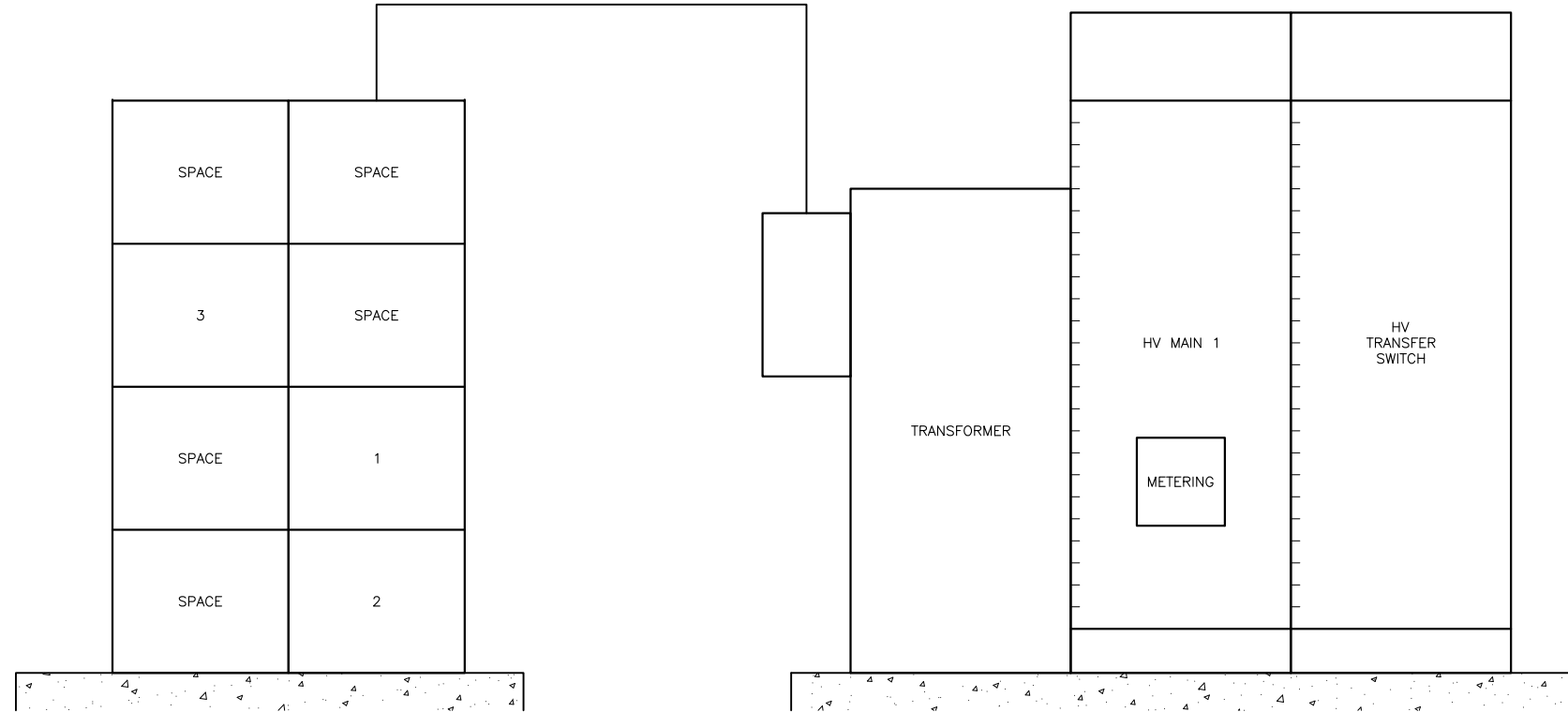
SUBSTATION 16 ELEVATION SCALE: NTS
